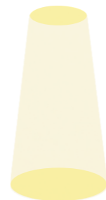
The light spot can be adjusted, from 9mm to 54mm under F250\text{mm} Objective lens
